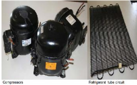
Picture 3. Compressors and refrigerant circuit. Note the labelling of compressors (white and orange labels)
