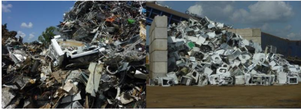
Picture 15. Left picture: pre-shredded material; Right picture: mono-flow
