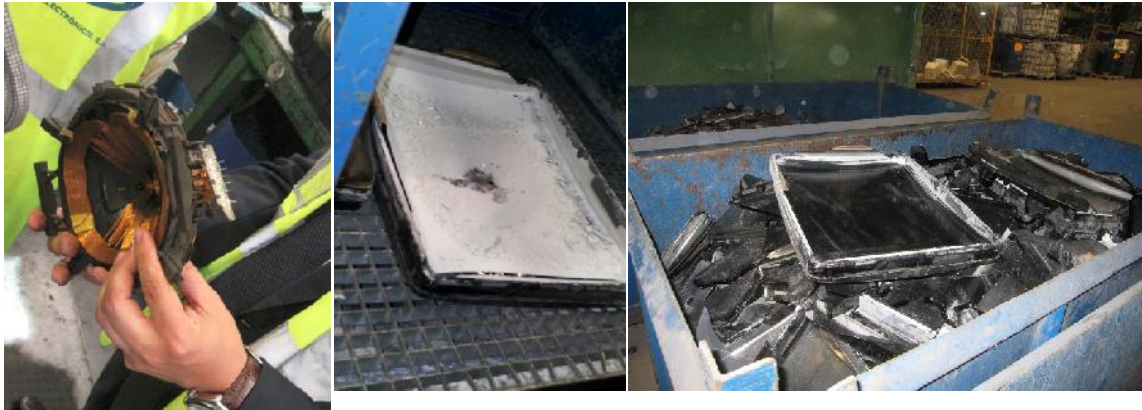
Picture 11. Left: Deflection coil from a CRT tube, the copper content of this component is highly appreciated by illegal collectors. Middle: uncleaned panel glass; right: cleaned panel glass.
