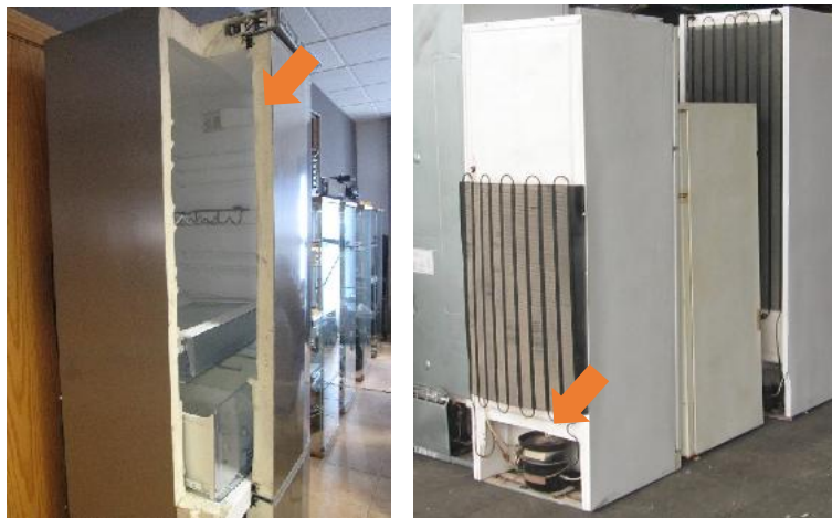
Picture 2. Left: detail of insulating foam in a fridge. Right: Location of a compressor in a fridge.
