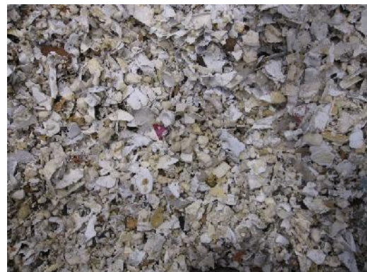
Picture 4. Fraction of shredded plastic from refrigerators. Pieces of insulating foam are visible in beige colour in the picture.
